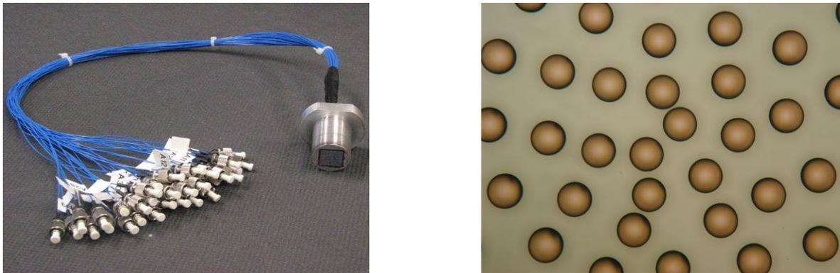
**Figure 5:** Aperiodic Optical Fiber array (left) and Aperiodic microlens array (right).
