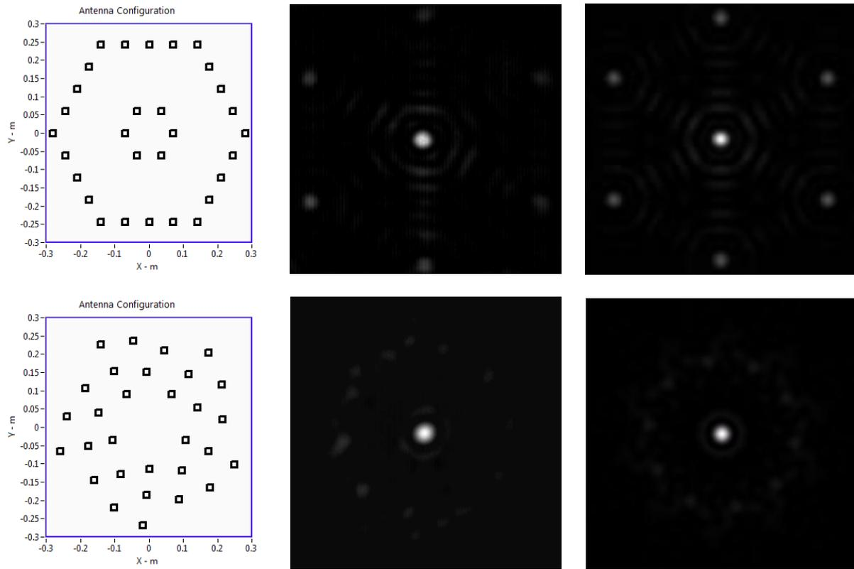
**Figure 7:** Antenna array configuration (left), measured point spread function (middle), and simulated point spread function (right). The upper row corresponds to the Pathfinder I, while the lower row corresponds to Pathfinder II.
