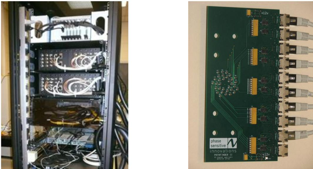
**Figure 3:** Rack mounted FPGA and distribution system (left) and Discrete Detector Receiver Board (right).
