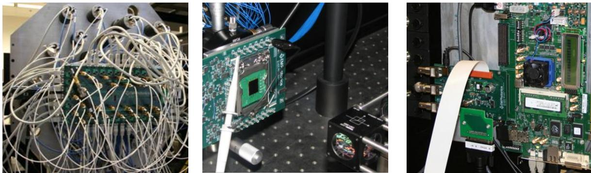
**Figure 4:** New Distribution Board attached to antenna array (left), FPA Receiver Board (middle), and FPGA Board (right).
