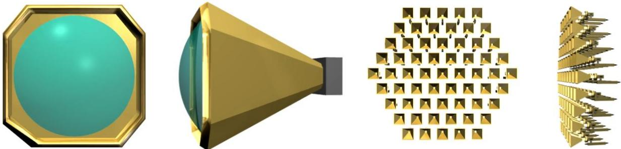
**Figure 1:** Three-dimensional form factor for a conventional imager relying on refractive optics and a focal plane array (front and side view, left) and an essentially two-dimensional form-factor for a distributed aperture imager with comparable aperture size and hence resolution capability (front and side view, right).
